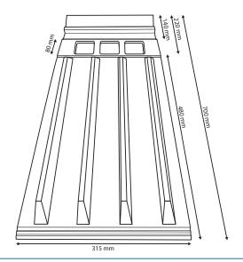
The Loft Vent Tray is easily installed from inside the loft to allow air into the roof space by preventing insulation material from blocking the ventilation path.
